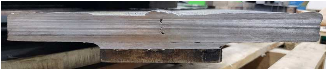
Fig. 3.4 Angular distortion measurement of constrained weld
