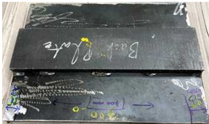
(b) steel backing condition of constrained weld
