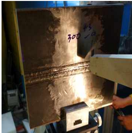
Fig. 3.17 Neutron diffraction measurement of constrained weld specimen
