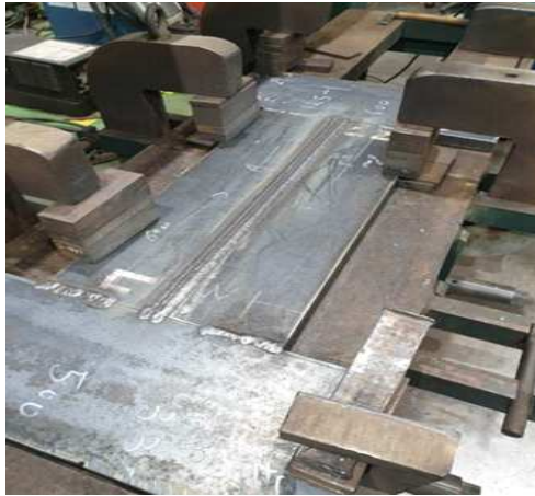
(a) constrained condition of constrained weld
