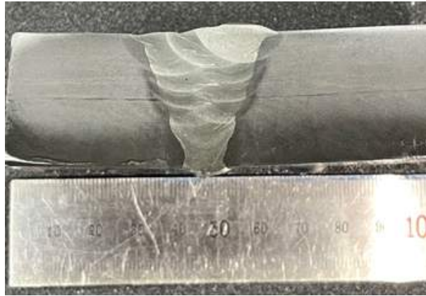
Fig. 3.3 Macrostructure of constrained weld specimen
