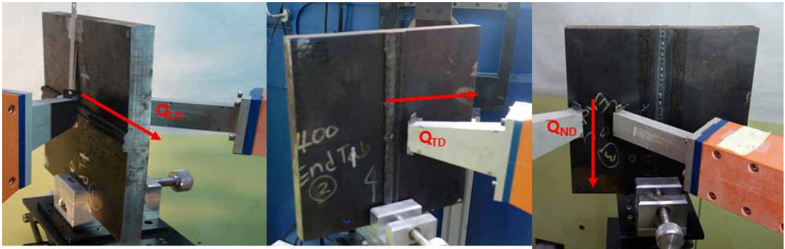
Fig. 3.41 Unconstrained weld specimen by neutron diffraction process
