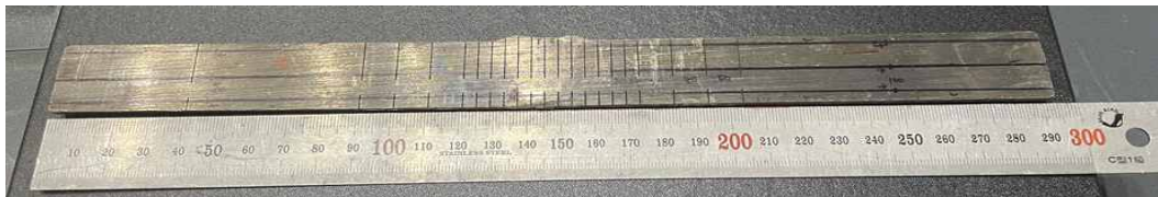
Fig. 3.18 Neutron diffraction measurement of constrained weld free specimen
