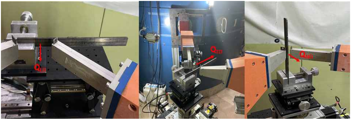
Fig. 3.21 Constrained weld stress free specimen contour method process
