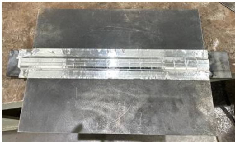
(b) ceramic backing condition of Unconstrained weld
