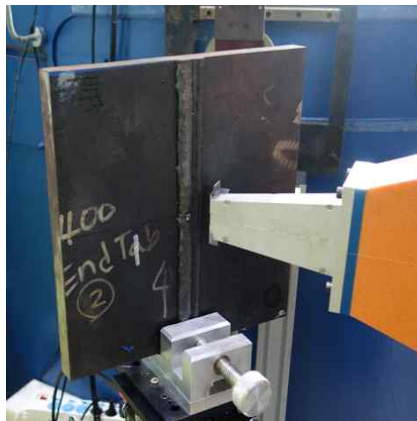
Fig. 3.38 Neutron diffraction measurement of unconstrained weld specimen
