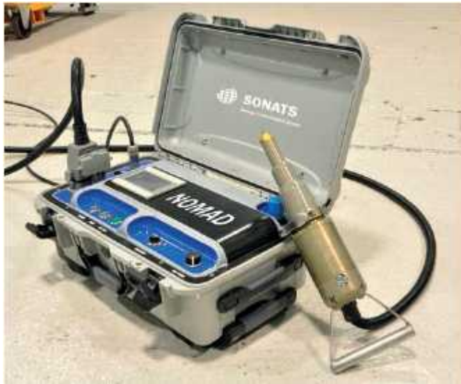
Fig. 3. 3. Ultrasonic peening equipment[28].
