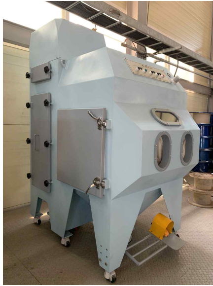
Fig. 3. 1. Shot peening equipment.
