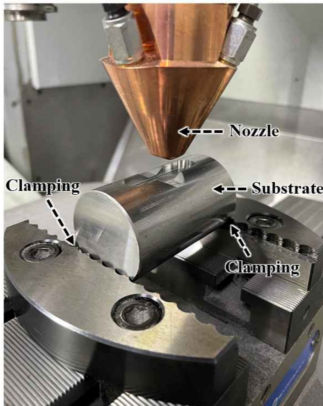
Fig. 100 Set-up for the deposition (repair experiments)
