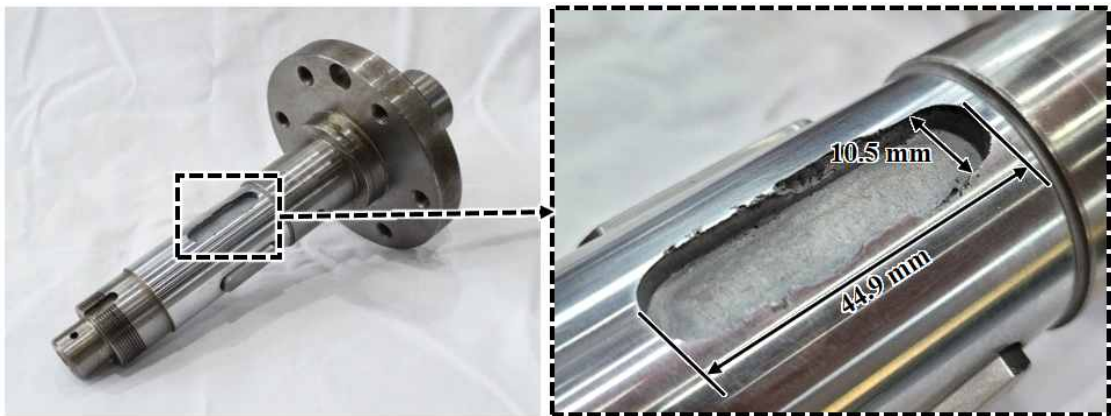
Fig. 97 The damaged parts of the shaft
