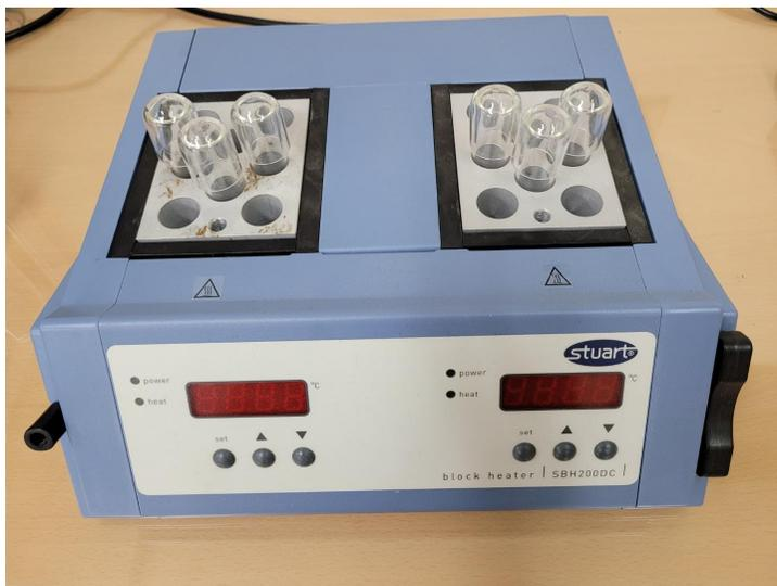
Fig. 25. Block heater for heat treatment
