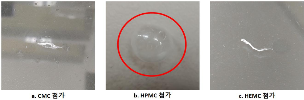
Fig. 27. Bubble film formation according to the cellulose derivatives. (a).bubble film of CMC solution. (b).bubble film of HPMC solution. (c).bubble film of HEMC solution.
