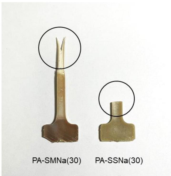
**Figure 13.** Fracture surface after tensile strength test of PA11 blends.
