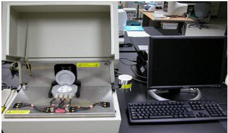
Fig. 13 Hall effect (Accent Optical Technologies. HL5500PC)
