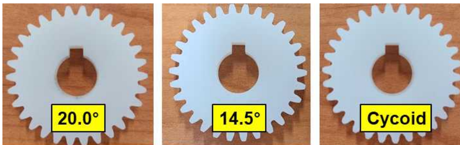
Figure. 11 Each gear specimens of different gear tooth shape
