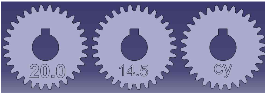
Figure. 10 Gear teeth profile drawing in Catia V5
