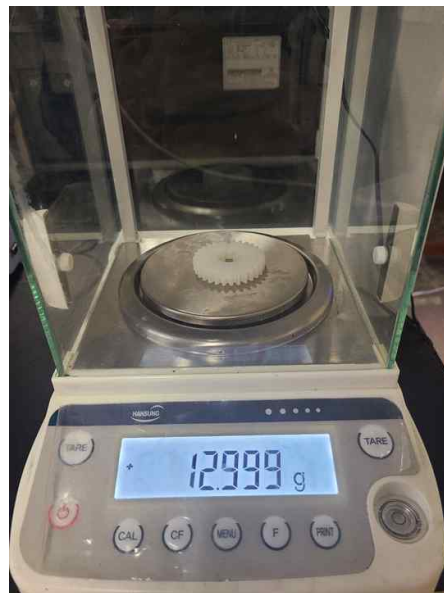
Figure. 15 Measuring weight loss after gear durability test for calculate wear rate
