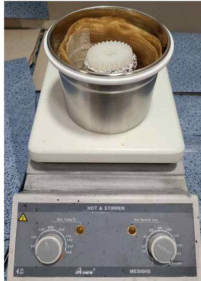
Figure. 27 Acetone fumigator for surface polishing
