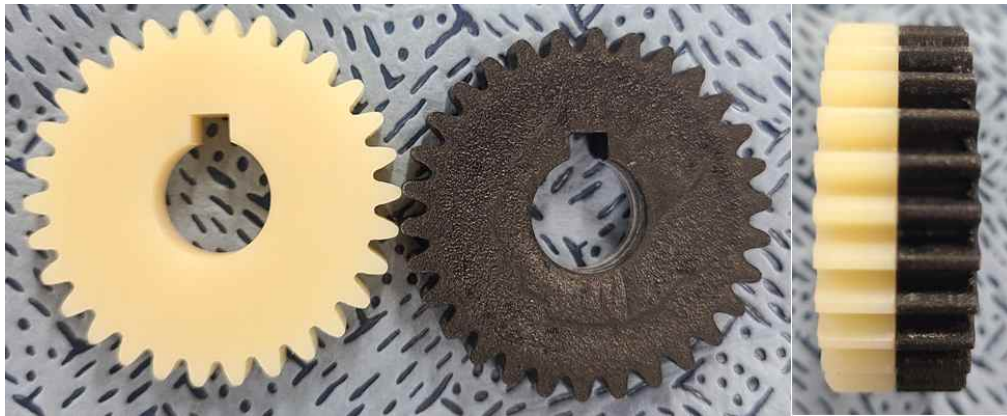
Figure. 43 PA12 polymer gear machining involute gear (left), CNT coated 3D printed cycloid polymer gear (right)
