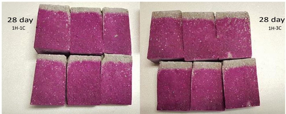
Figure 43: Phenolphthalein sprayed image of specimens
