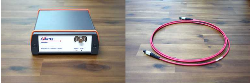
Figure 5.3. Gas species analyzing device. Optical emission spectrometer (left) and optical fiber (right).
