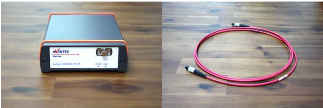
Figure 4.3. Gas species analyzing device. Optical emission spectrometer (left) and optical fiber (right).
