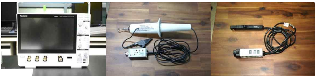
Figure 4.4. Device for analyzed electrical characteristics of plasma discharge. Oscilloscope (left) and high voltage probe (middle) and current probe (right).
