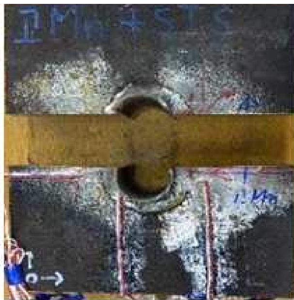
Fig. 2.5 Residual stress measurement after cutting
