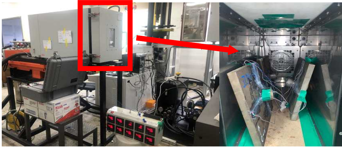
Fig. 3.1 Cooling chamber for specimen experiment
