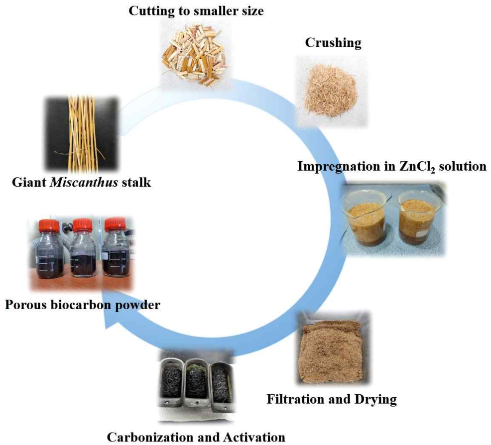
Figure 3.2. Flowchart for preparation of the porous biocarbons.
