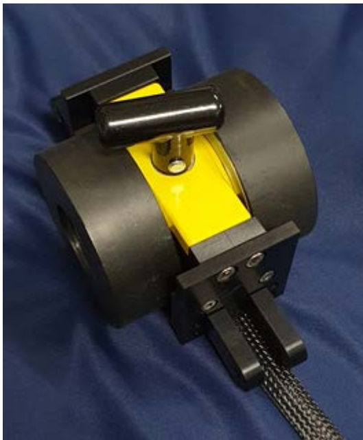
Fig. 5 -10 Prototype of magnetizer unit-1 and magnetizer unit-2
