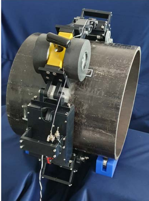
Fig. 5 -5 Prototype static balancing scanner for inspection of pipe welding
