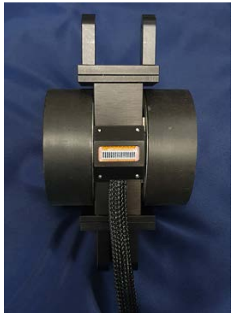
Fig. 5 -10 Prototype of magnetizer unit-1 and magnetizer unit-2
