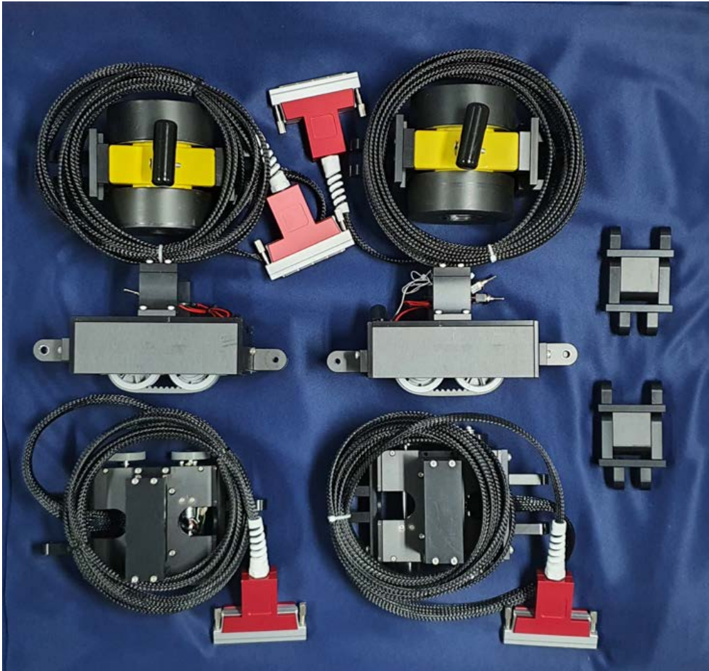
Fig. 5 -12 Overall configuration of static balancing scanner
