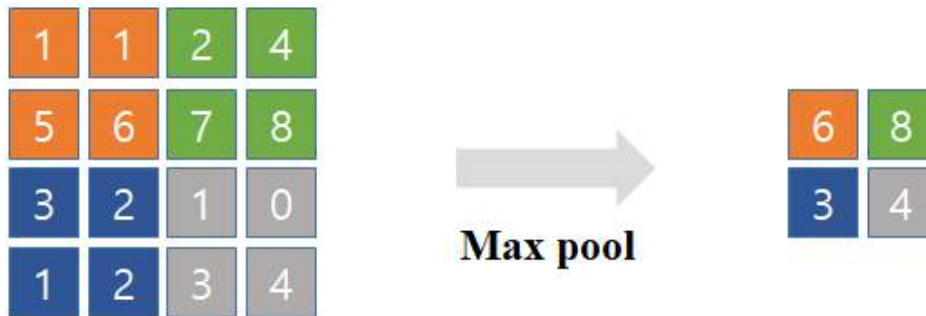
Figure 20. The example of max pooling operation
