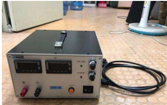
Fig. 2.10 Photograph of DC power supply
