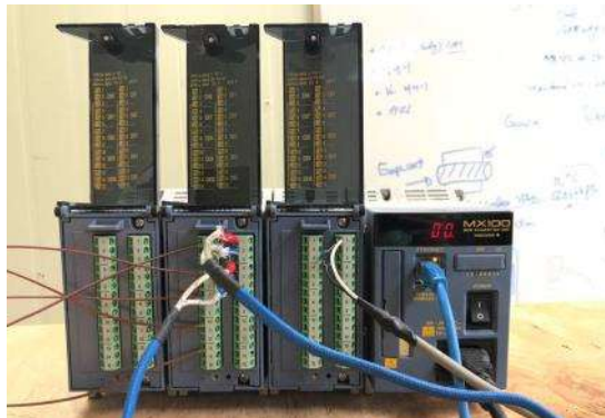
Fig. 2.12 Photograph of data acquisition system
