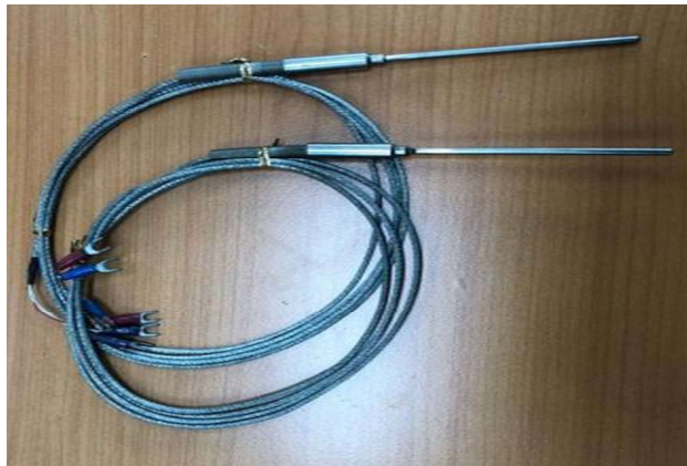
Fig. 2.5 Photograph of T-type thermocouple
