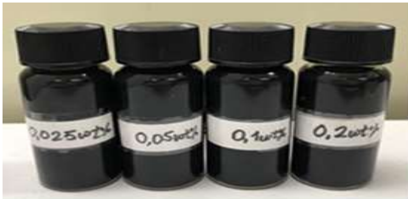
Fig. 2.17 Pictures of Fe 3 O 4 /MWCNT hybrid nanofluids
