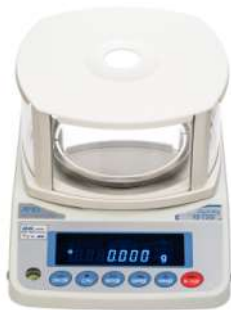
(a) Precision Balance (FX-300i)
