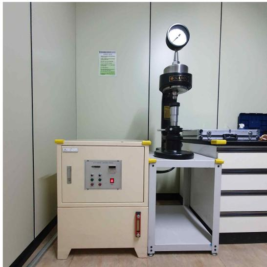
Fig. 3.7 Brinell hardness tester. (SB-700)
