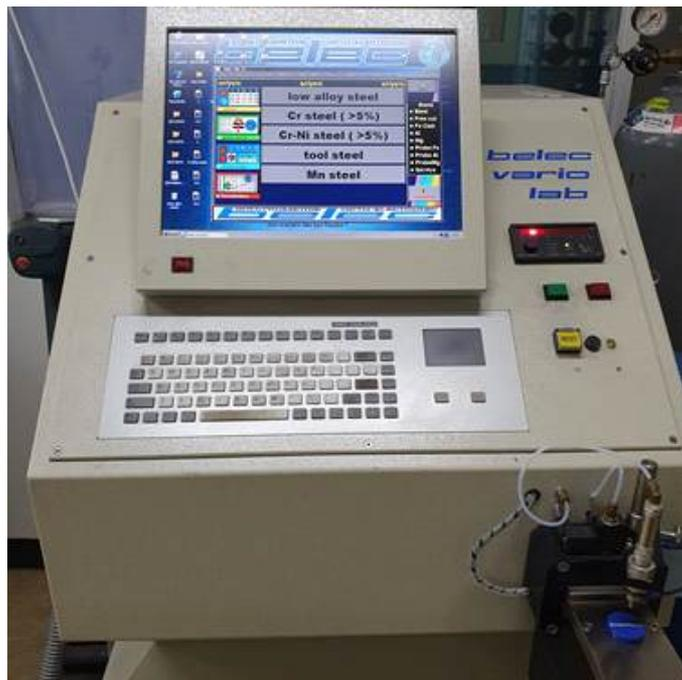
Fig. 3.2 Spark emission spectrometer. (Vario Lab, BELEC.)
