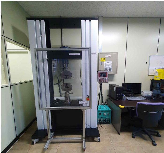
Fig. 3.5 Universal testing machine. (TO-102-300 kN)
