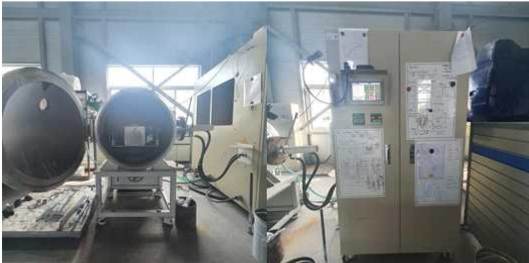
Fig. 3.1 High frequency induction melting furnace. (HF-50K, ELTek Co.)
