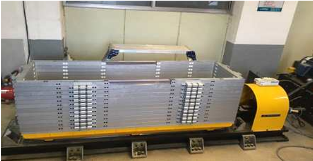
Fig 3.2 Laminar shear box used in this study.
