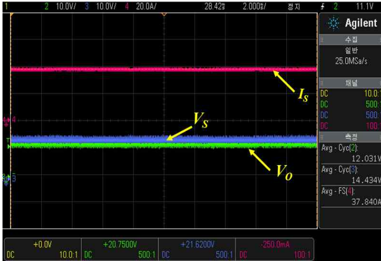
Fig. 5-17. Forward Measurement Result 1(Input) V_s=14.43[V]
