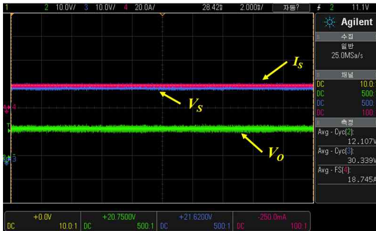
Fig. 5-21. Forward Measurement Result 5(Input) V_s=30.33[V]
