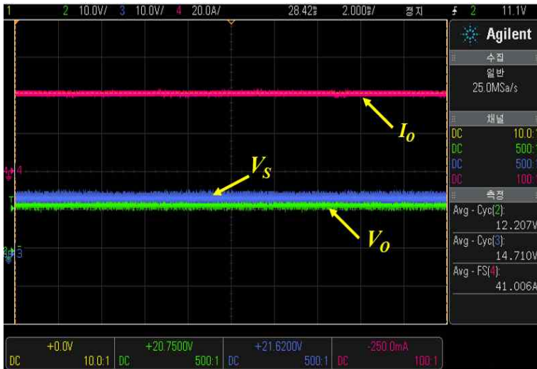
Fig. 5-18. Forward Measurement Result 2(Output) V_o=12.20[V]
