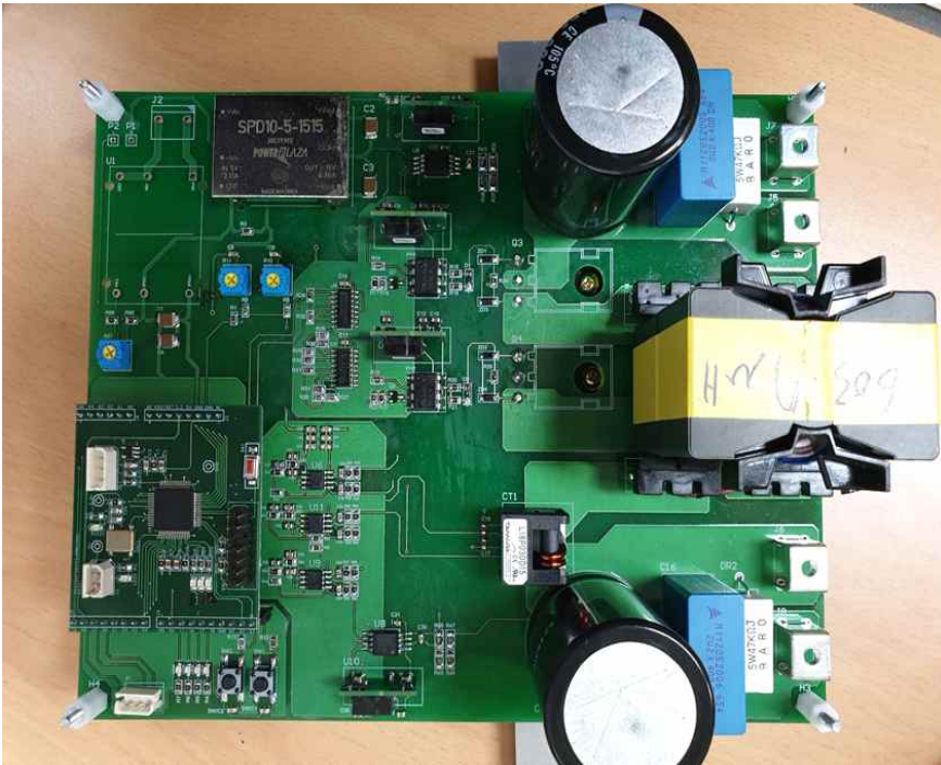
Fig. 5-7. 500[W] Class MPPT Battery Charging Converter
