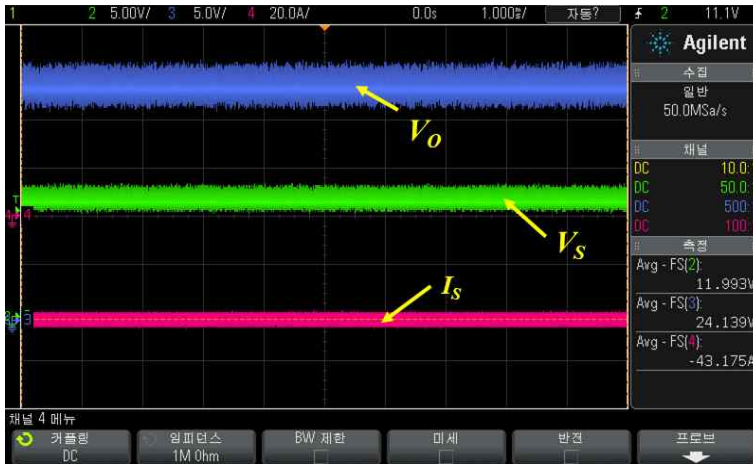
Fig. 5-23. Reverse Measurement Result 1(Input) I_{IN} = -43.17[A]
