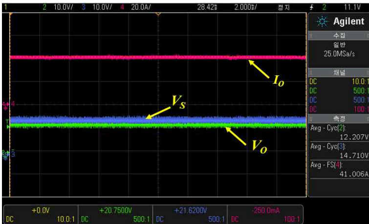
Fig. 5-22. Forward Measurement Result 6(Output) V_o=12.20[V]
