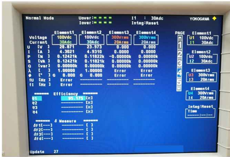
Fig. 5-25. Converter Maximum Efficiency Measurement Screen
