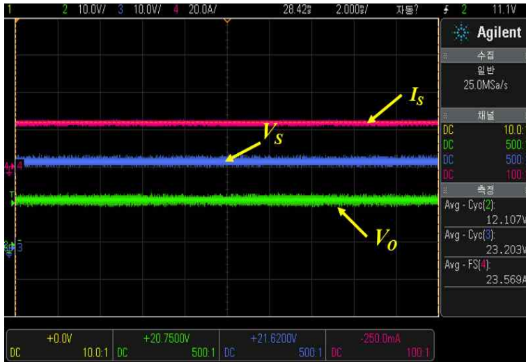
Fig. 5-19. Forward Measurement Result 3(Input) V_s=23.20[V]
