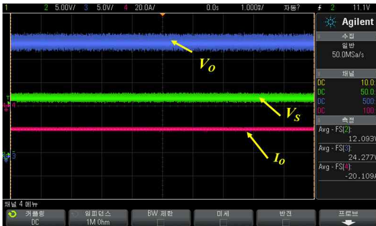
Fig. 5-24. Reverse Measurement Result 2(Output) I_{IN} = -20.10[A]
