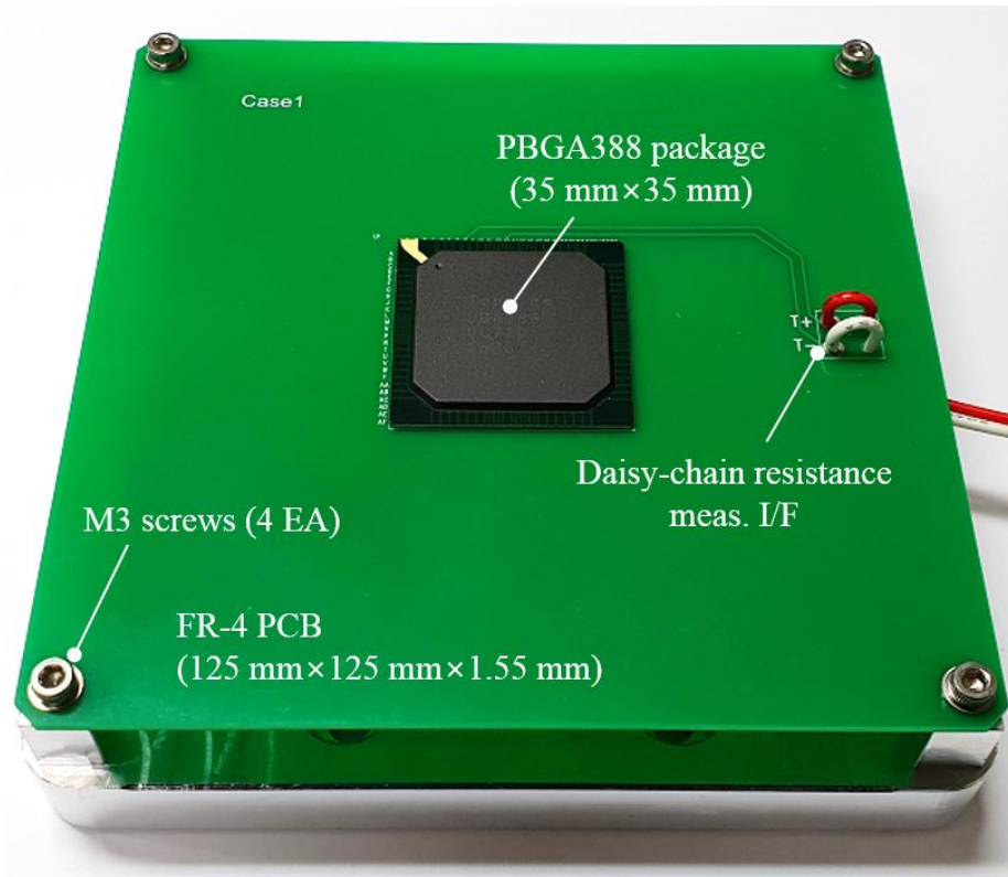
Fig. IV-3 Representative configuration of sample PCB assembly in Case 1
