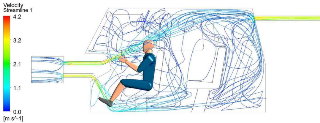
(b) Simulation velocity streamline (this study)
