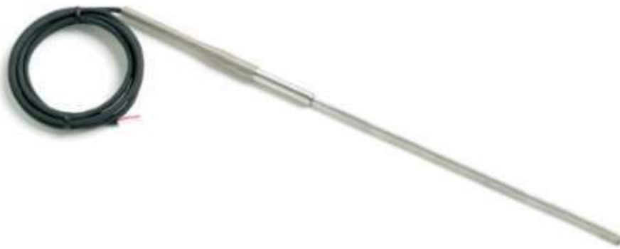
Fig. 4.12 Photograph of T-type thermocouple
