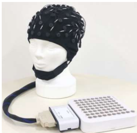
Fig. 4.8 Electroencephalogram measuring equipment
