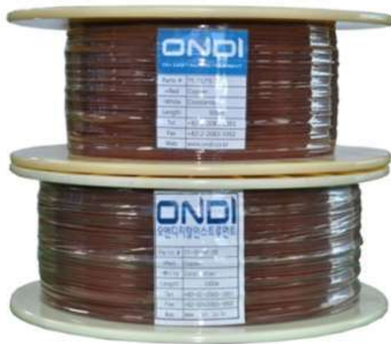
Fig. 4.13 Photograph for the wire form of T-type thermocouple
