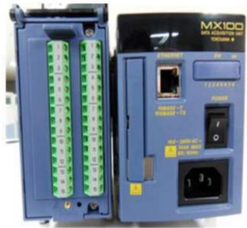
Fig. 4.16 Photograph of data acquisition system
