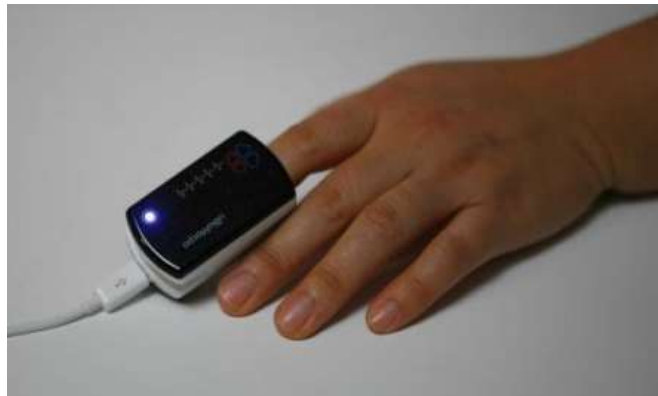
Fig. 4.7 Experimental device to measure PPG
