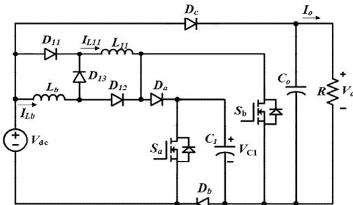
Figure 1. High Gain DC-to-DC Boost Type Converter.
