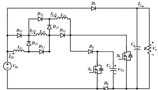
Figure 2. Proposed High Gain DC-to-DC Boost Type Converter employing 2 switched-inductor cell.
