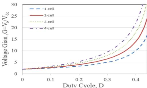
Figure 6. Comparative plots of voltage gain and duty cycle with employing n-switched-inductor cells.
