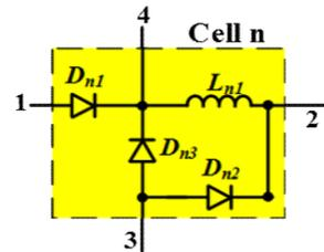
Figure 4. The structure of a switched-inductor cell.
