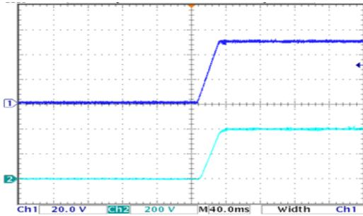
Figure 8. Dynamic performance of high gain DC-to-DC boost type converter employing 1 switched-inductor cell. From top to bottom: input voltage and output voltage.
