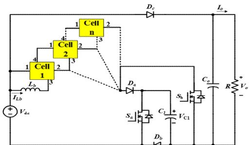
Figure 5. Proposed Converter employing Multi switched-inductor cells
