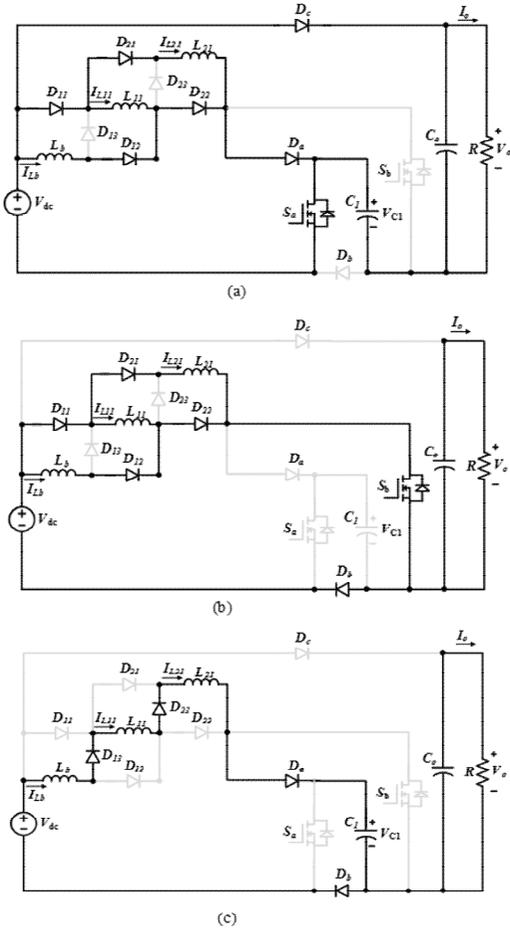
Figure 3. Operating states of the proposed converter: (a) state 1, (b) state 2, and (c) state 3.
