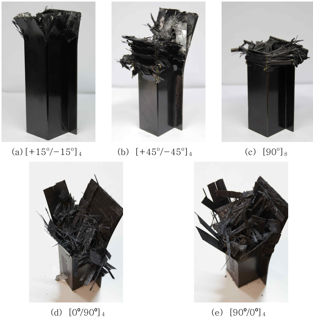
Photo. 4 Collapsed shape of CFRP hat-shaped sectional members ( dry specimen)
