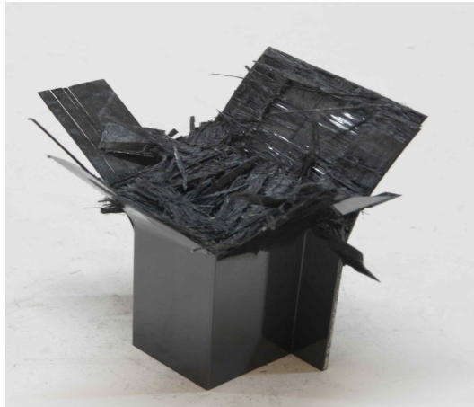
(a) Collapse shape
