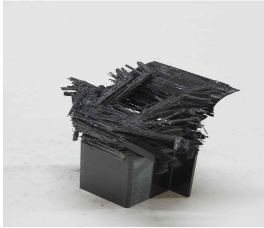
(a) Collapse shape
