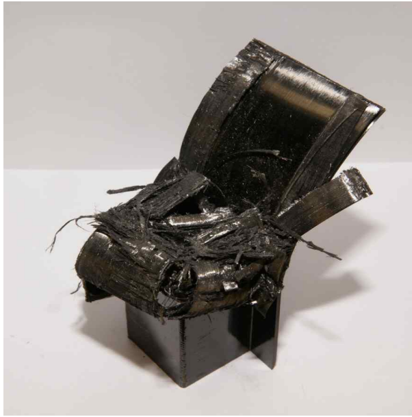
Photo. 10 Collapsed shape of CFRP hat-shaped sectional members ( dry specimen, 7 interface, outer angle 90°, Static)
