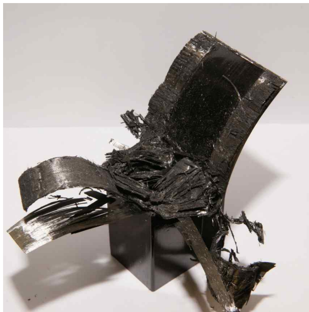
Photo. 11 Collapsed shape of CFRP hat-shaped sectional members ( dry specimen, 7 interface, outer angle 0°, Static)
