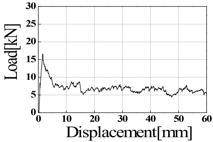
Fig. 21 Load–displacement curve of CFRP single hat shaped member, [0_2/90_2]_s ( 2 interface number)
