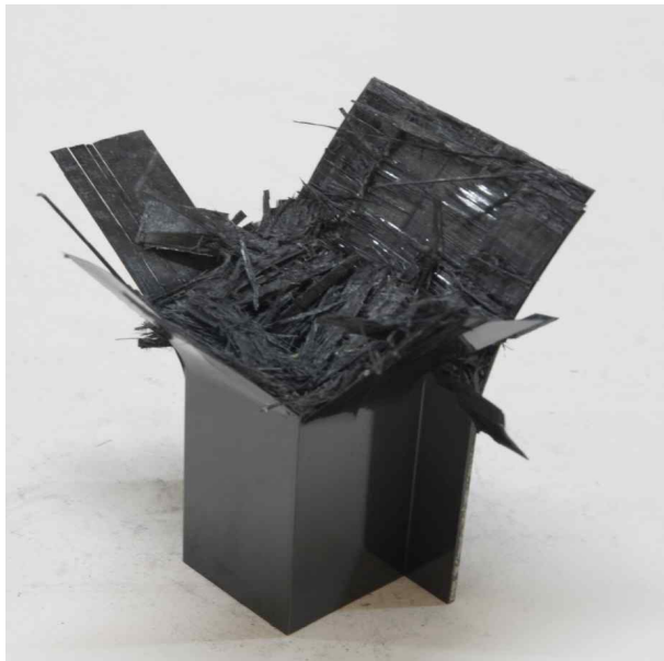
Photo. 15 Collapsed shape of CFRP hat-shaped sectional members ( wet specimen, 7 interface, outer angle 0°, Impact )
