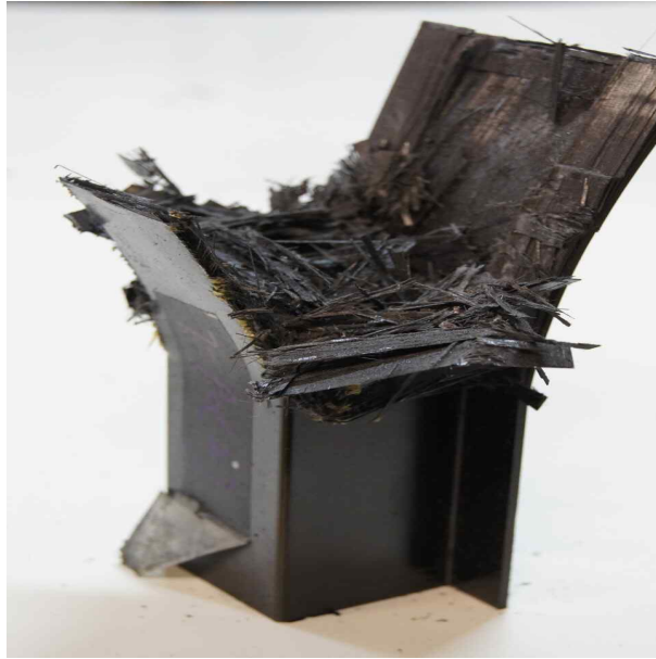
Photo. 12 Collapsed shape of CFRP hat-shaped sectional members ( dry specimen, 7 interface, outer angle 90°, Impact )
