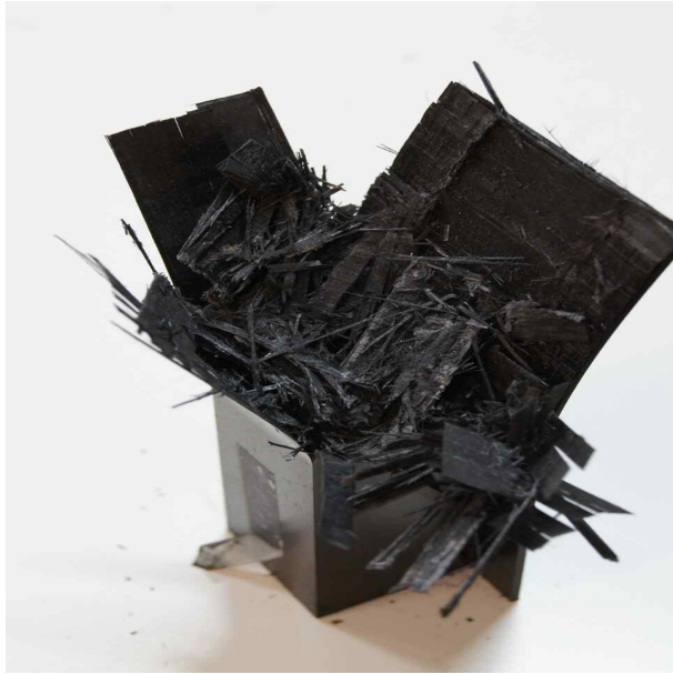
Photo. 14 Collapsed shape of CFRP hat-shaped sectional members ( dry specimen, 7 interface, outer angle 0°, Impact )
