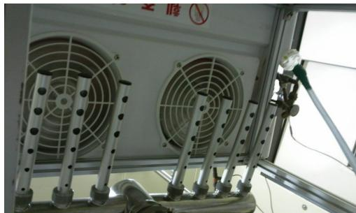
Fig. 3.5 Air sampler indoor side.
