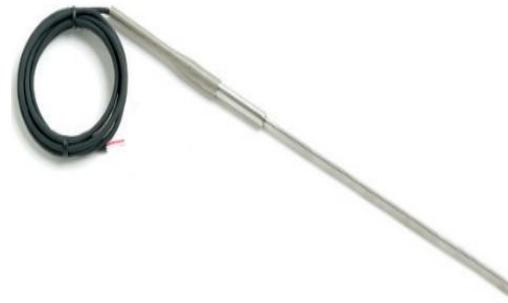
Fig. 3.15 Photograph of T-Type Thermocouple.
