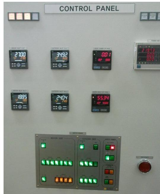
Fig. 3.4 Control panel of psychrometric chamber.
