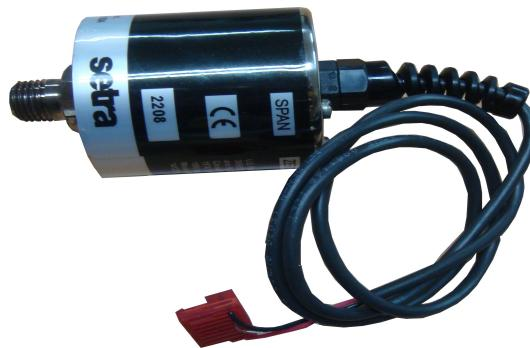
Fig. 3.14 Photograph of pressure gauge.
