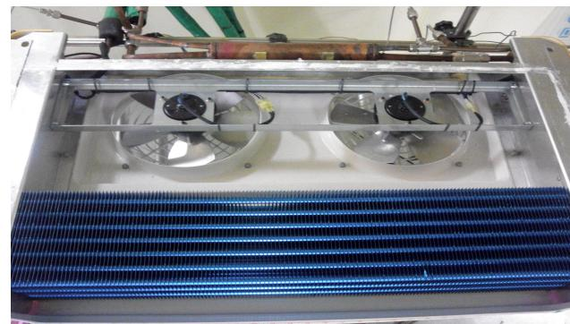
Fig. 3.13 Photograph of evaporator.
