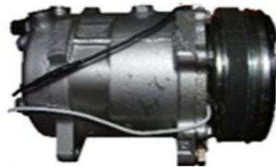
Fig. 3.9 Photograph of Swash plate compressor.
