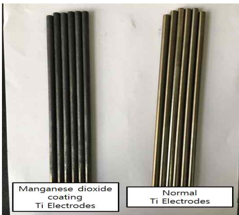
Figure 2 Manganese coated titanium electrode and normal titanium electrode.
