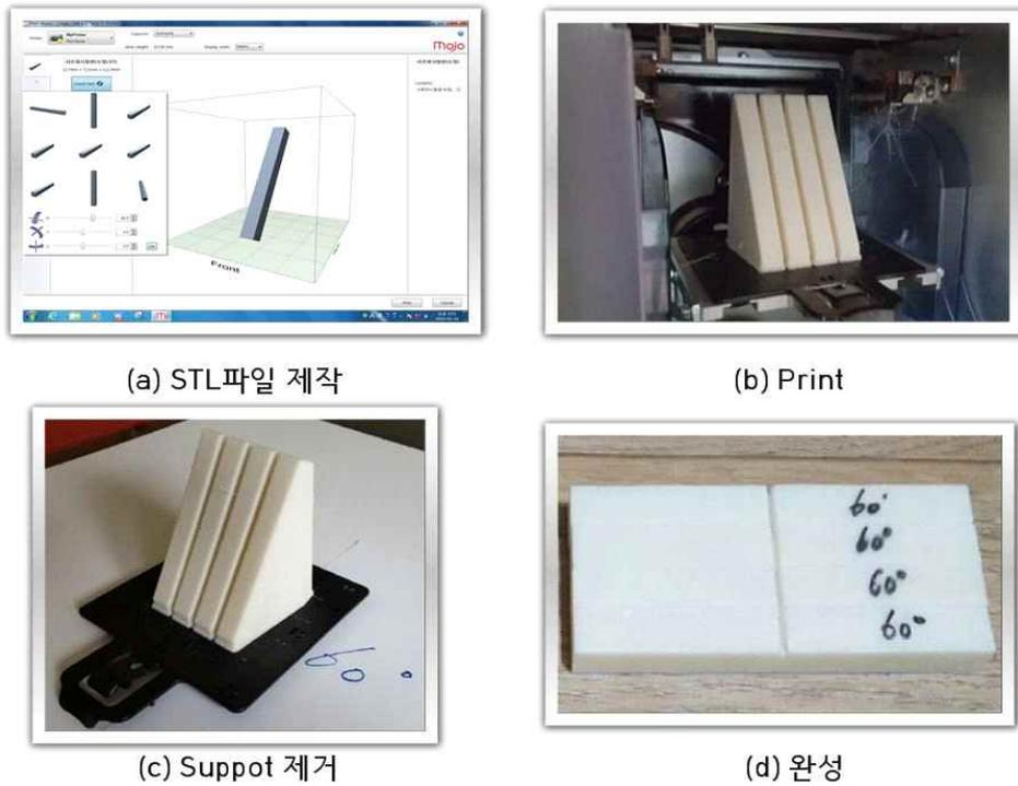
Fig. 24 Charpy impact Specimen production process(60°)
