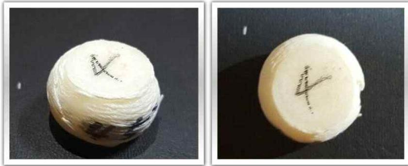
Fig. 33 Specimen compression fracture state(45°)
