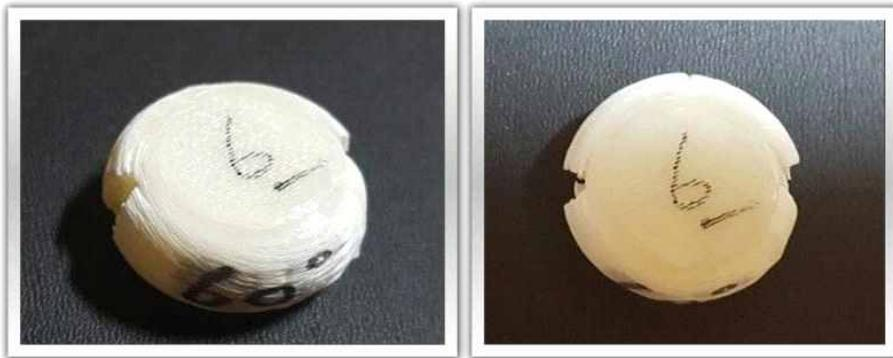
Fig. 34 Specimen compression fracture state(60°)
