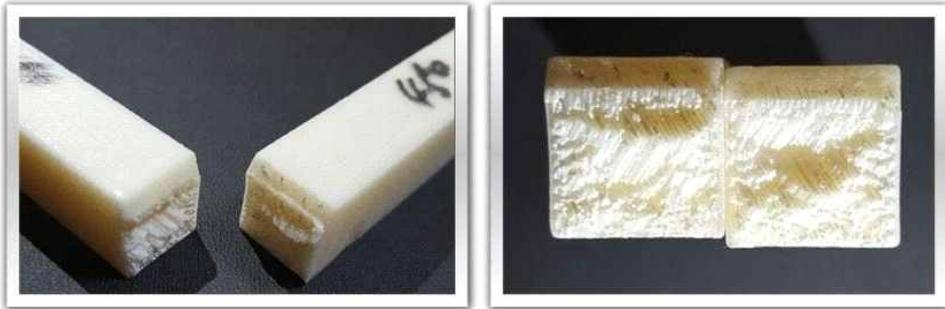
Fig. 40 Specimen impact fracture state(45°)
