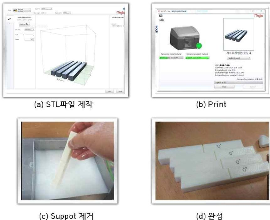
Fig. 21 Charpy impact Specimen production process( $0^\circ$ )
