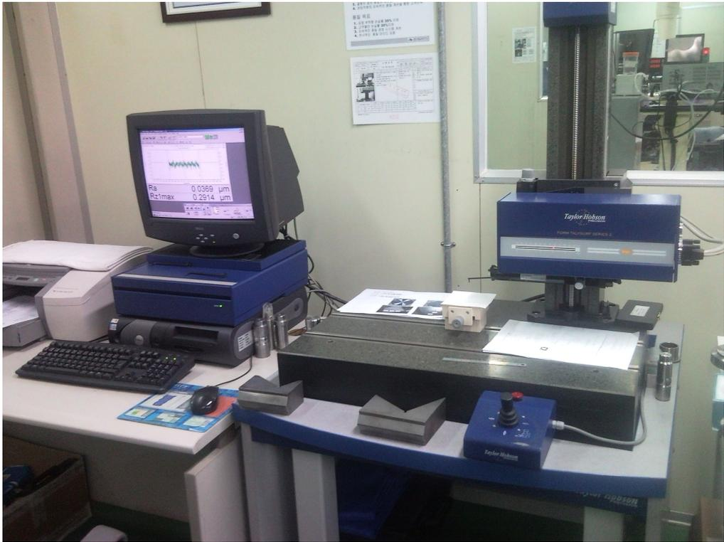
Photo. 3.2 Surface roughness tester (Taylsurf PGI 800)
