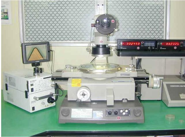
Photo. 3.4 Tool maker's microscope
