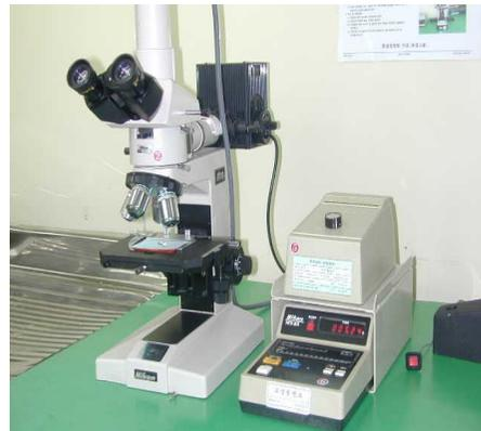
Photo. 3.3 Metallurgical microscope
