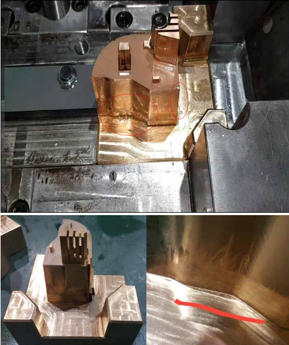
Fig 1.1 Water leak due to crack in the corner part on hot spot of plastic parts
