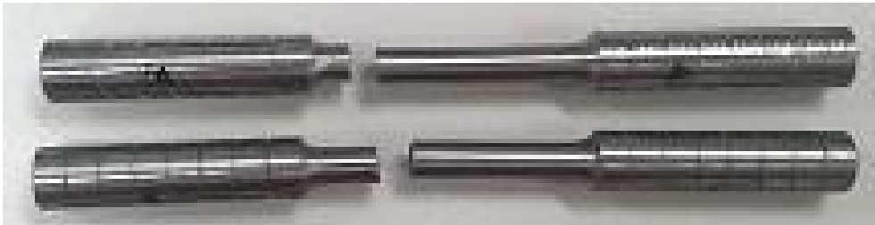
Fig 2.7 Stand specimen for tensile test(product)
