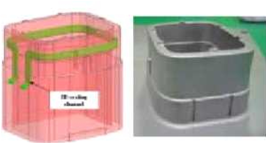
Fig 1.2 Three-dimensional cooling channel in core insert and core insert produced by DMLS process [1]
