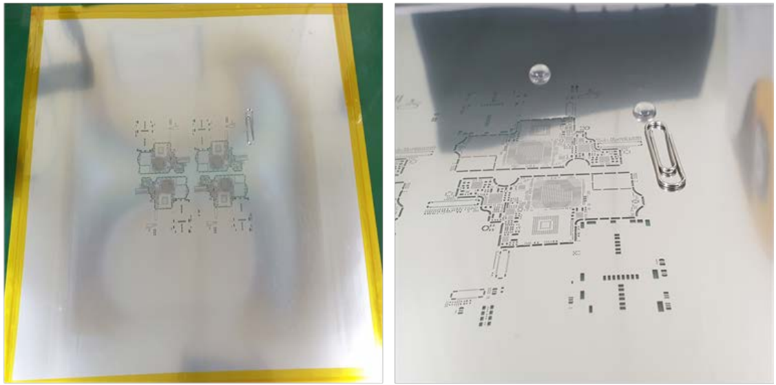
Fig. 4-18 Copolymer applied stencil digital image.
