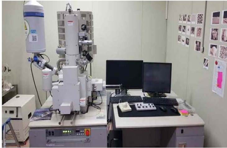
Fig. 4-12 Surface morphology measurement device SEM
