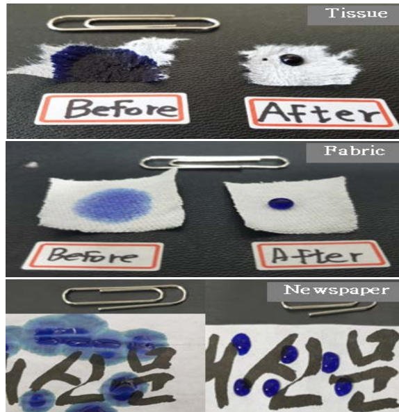
Fig. 4-2 Hydrophobic thin film Coating image. (Tissue, Fabric, Newspaper)
