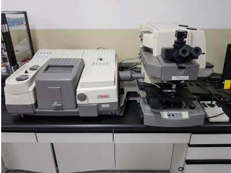
Fig. 4-10 Chemical structure & composition analysis device FT-IR
