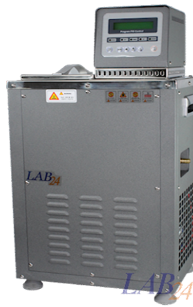
Fig. 2.11 Low temperature water bath (RBC-08)
