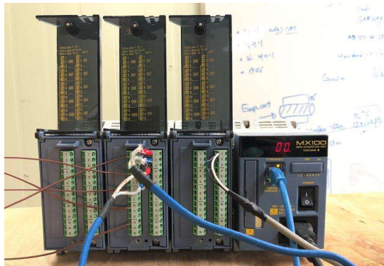
Fig. 2.15 Data acquisition system (MX100)
