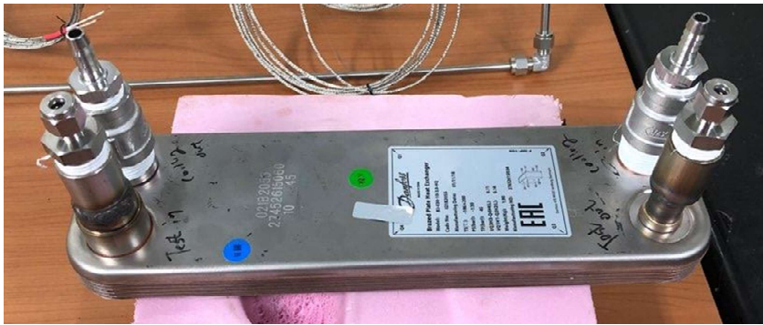
Fig. 2.8 Brazed plate heat exchanger (B3-030-10-3.0-HQ)
