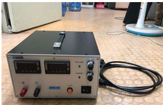
Fig. 2.10 DC power supply (DSP-2005)
