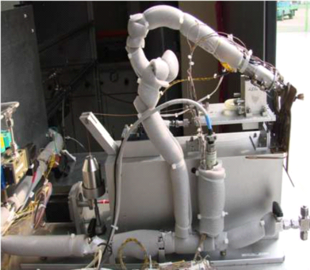
Fig. 16 HAN based propellant performance evaluation
