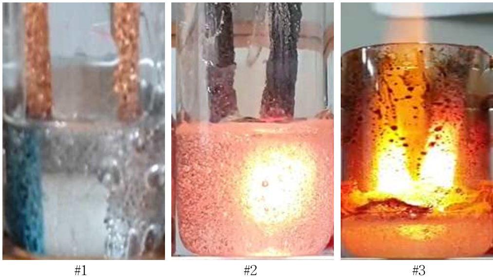
Fig. 2.14 Behavior of gelled HAN propellant electrolytic ignition with copper foam; #1 : Initial reaction with electrode, #2 : Initiation of ignition, #3 : Ignition without power input; Left side electrode is cathode(+), right side electrode is anode(-)
