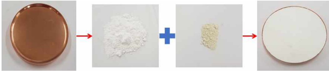
Fig. 2 Photograph illustrates the sequence to produce the \text{Ga}_2\text{O}_3+\text{SnO}_2 powder target.
