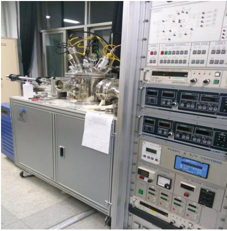
Fig. 9. RF magnetron co-sputter(I.D.T. ENG.)
