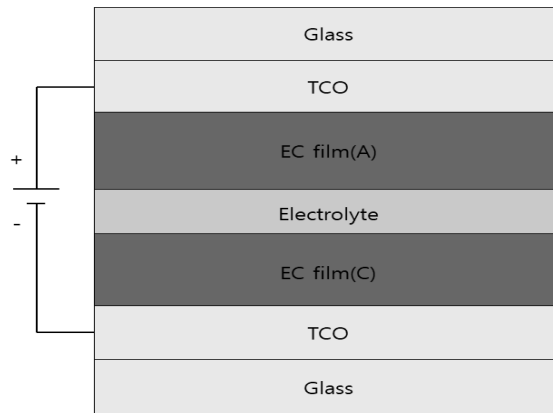
Fig. 1. Structure of Electrochromic Device
