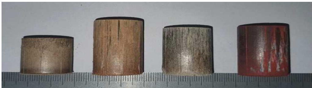
1. Bentonite 2. Soil sludge 3. Concrete sludge 4. Sump sludge
