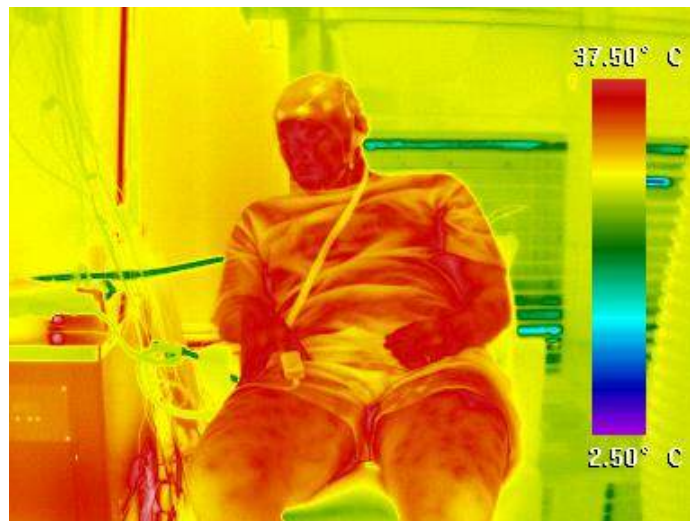
Fig. 4.19 Surface temperature in the using cold water cooling seat under 27.5°C condition
