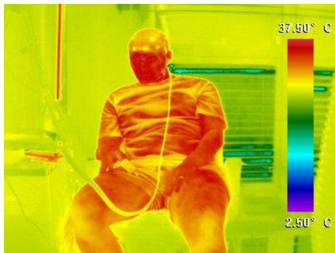
Fig 4.14 Surface temperature results in the ventilation seat under 27.5°C condition
