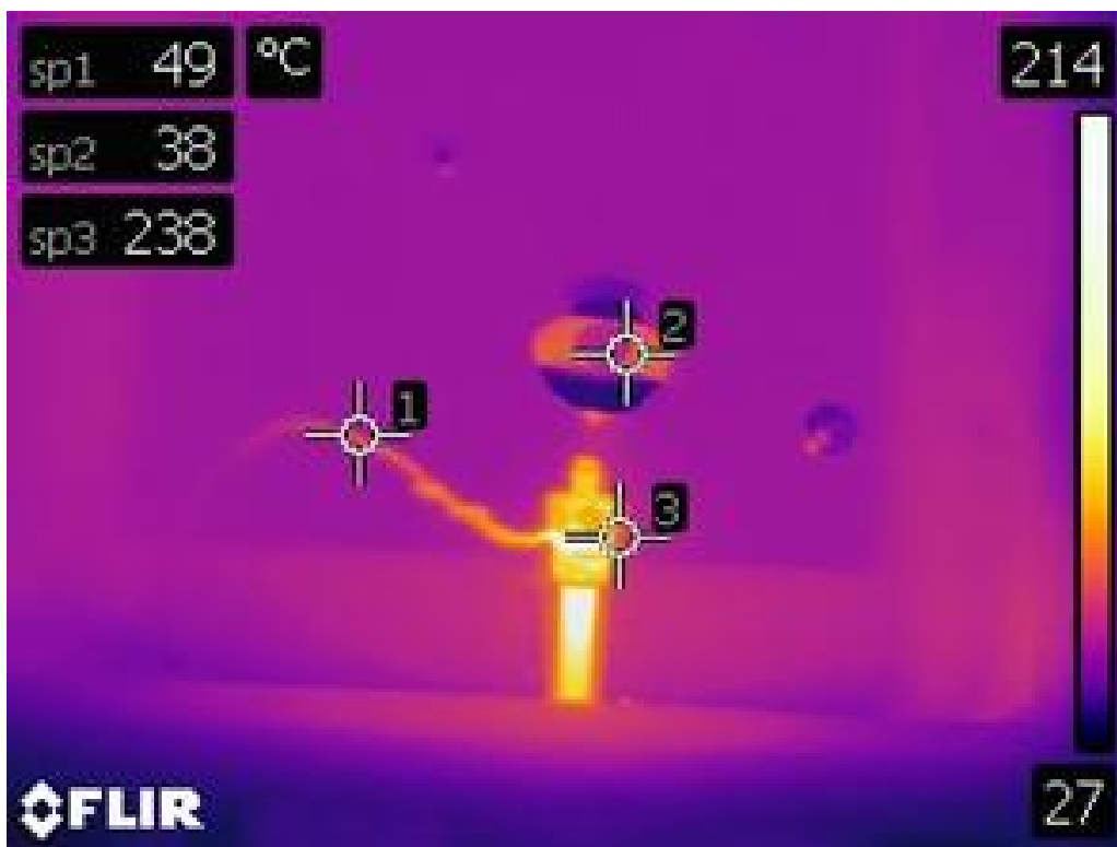
Fig. 26 The temperature of plasma nozzle and sample in the DRIFTS apparatus.
