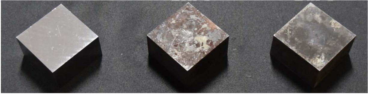
(a) Without heat treatment (b) With heat treatment at 500 °C (c) With heat treatment at 400 °C
