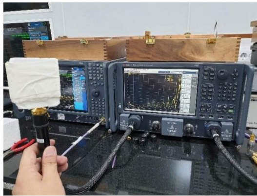
Figure 5.2. Measurement set up of the prototype antenna
