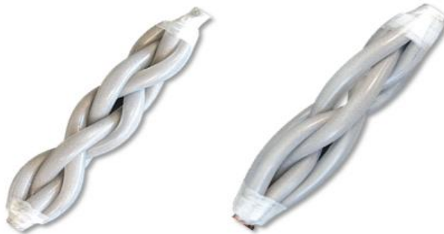
Figure. 9-3 Quadruple and quintuple structured CCTENGs.
