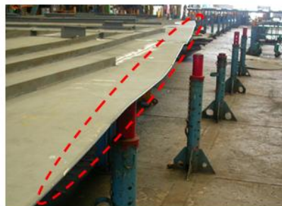
Fig. 1.1 Welding distortion in ship-yard
