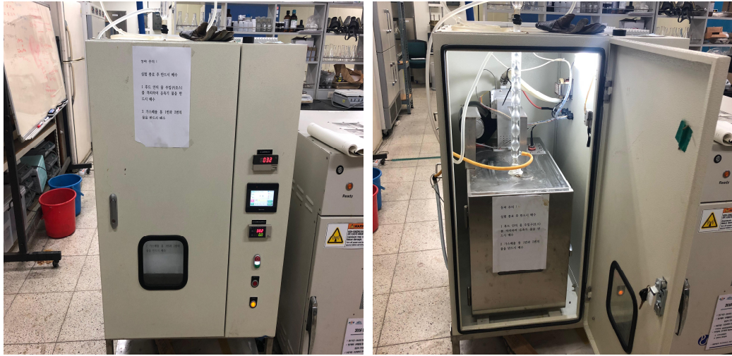
Fig. 3-4 The photograph of microwave equipment for nitric acid leaching.
