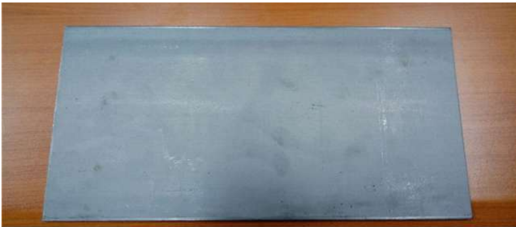
Fig. 3-19 Panel specimen for measuring change of temperature by high frequency induction heating for 8 sec of heating time
