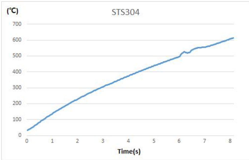
Fig. 4-14 Graph of temperature change on the surface of STS304 panel heated by high frequency induction heating device
