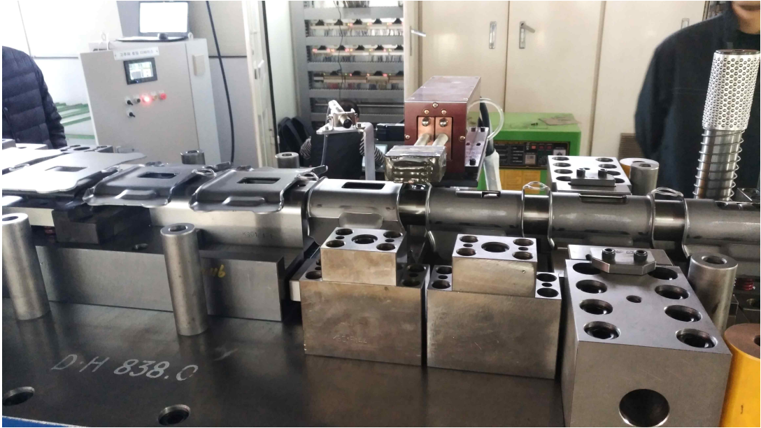
Fig. 3-13 Practical use of high frequency induction heating device for producing knuckle bracket
