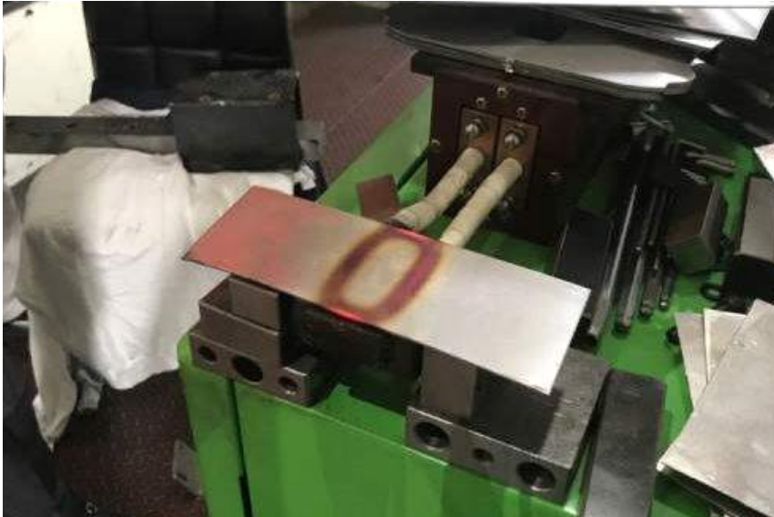
Fig. 3-20 Experiment for heating panel specimen using high frequency induction heating device
