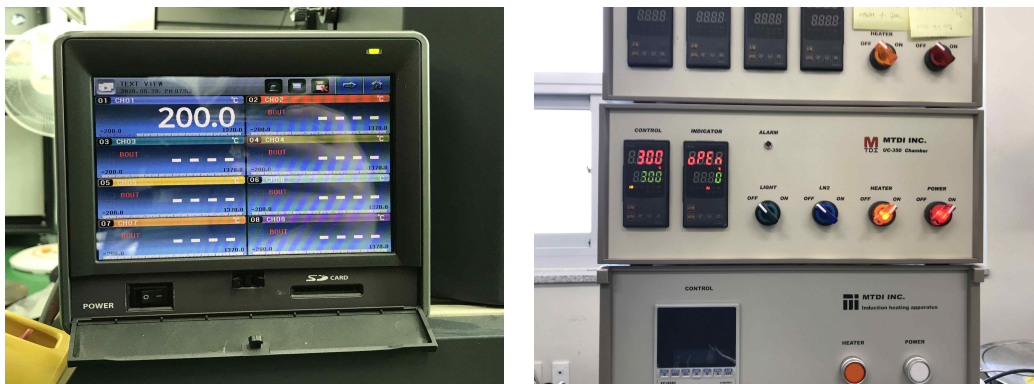
Fig. 3-18 Temperature control device for tensile testing under high temperature
