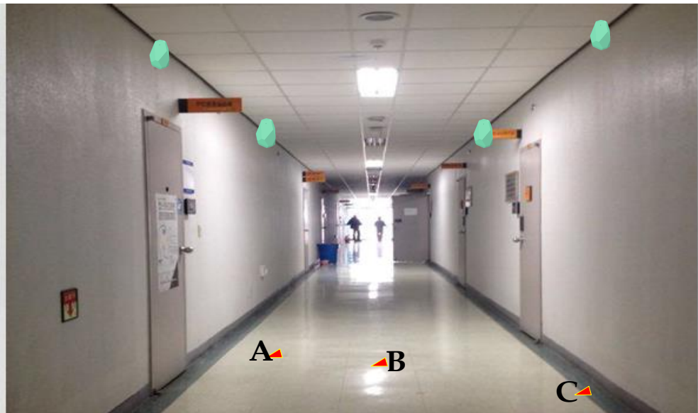
Figure 4.7: Experimental environment: beacons deployed in the corridor where measurement places are marked on the floor as A, B, and C.
