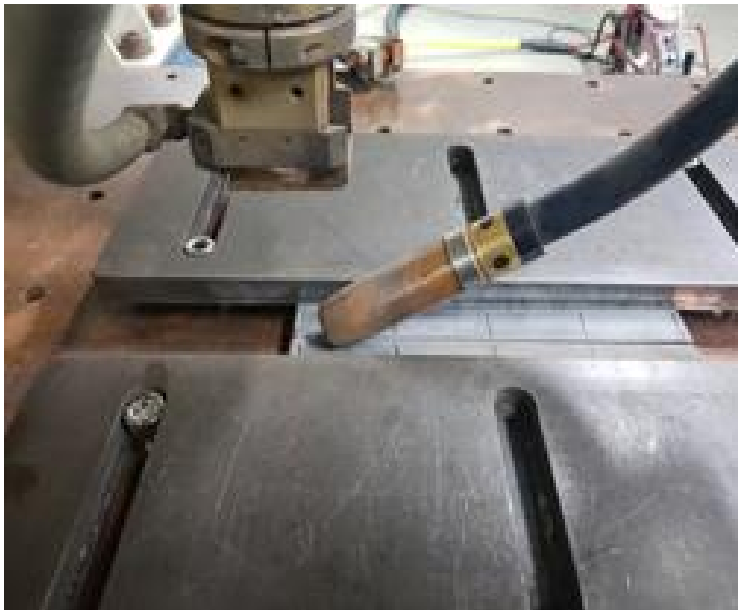
Fig. 3.1 Prevention device of laser-arc hybrid welding deformation
