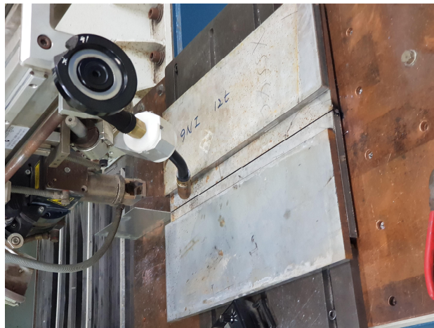
Fig. 3.2 Laser-arc hybrid welded specimen for destructive test
