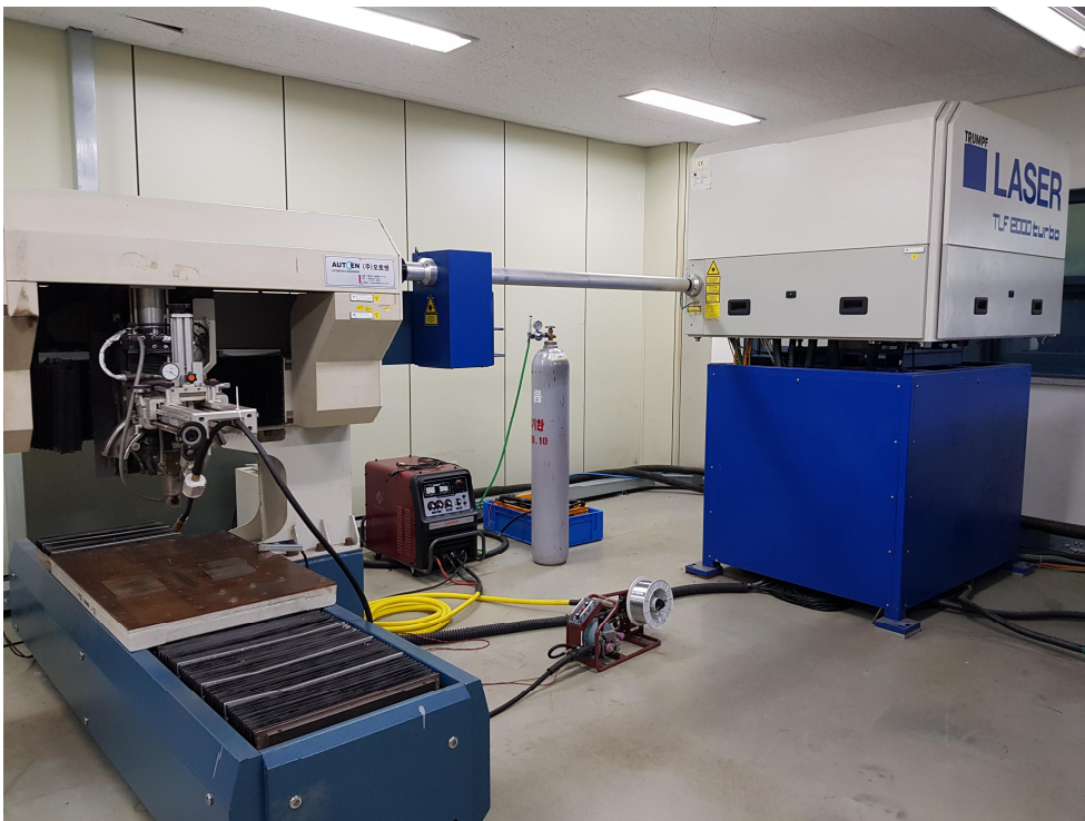
Fig. 2.1 Experimental setup for CO 2 laser-GMA hybrid welding system
