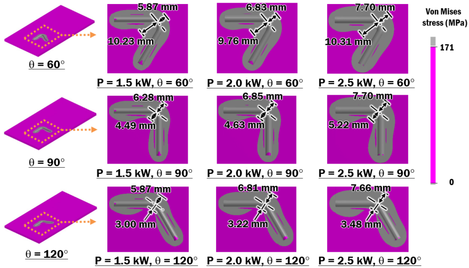
Fig. 51 Formation of SIR according to power of laser and angle of corner deposition 88
