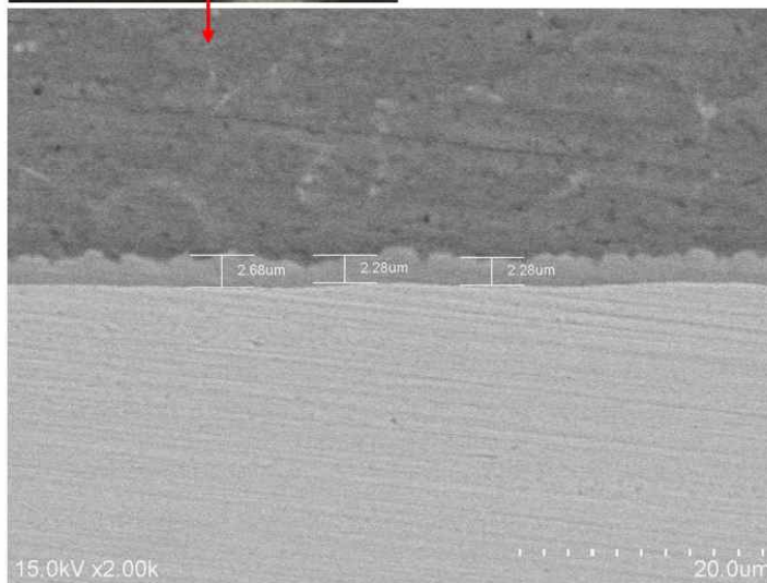
Fig. 3.2 Thickness of Intermetallic Compound by EN Ratio
