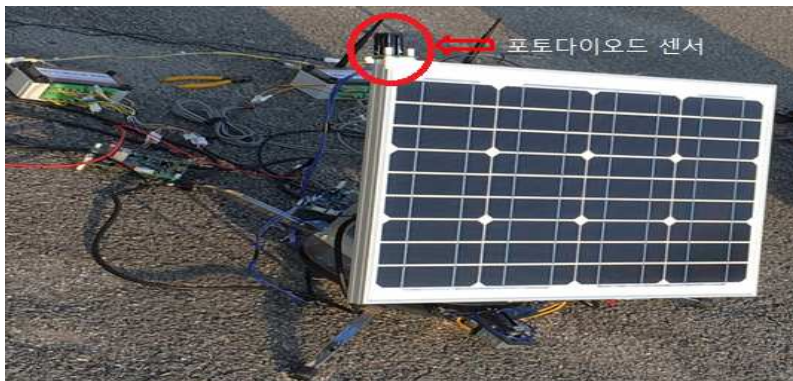
Fig. 11. Diagram of tracking PV system
