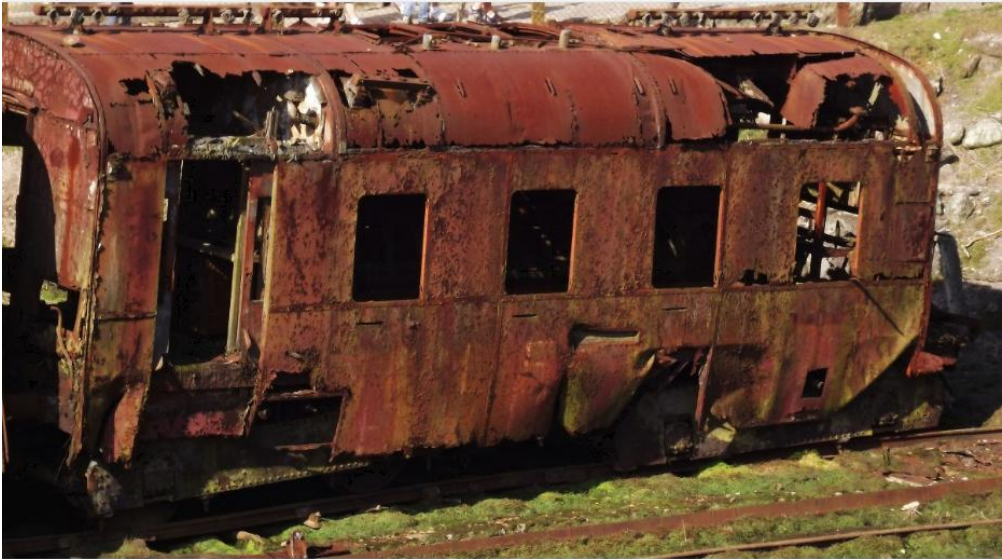
Figure 2.1 Train with uniform corrosion
