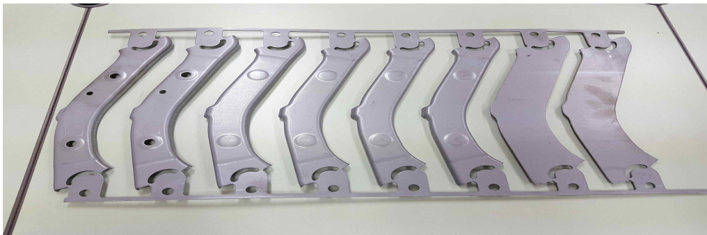
Fig. 1.5 Products of progressive mold
