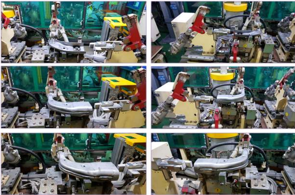
Fig. 2.2 Lower and upper assy jig
